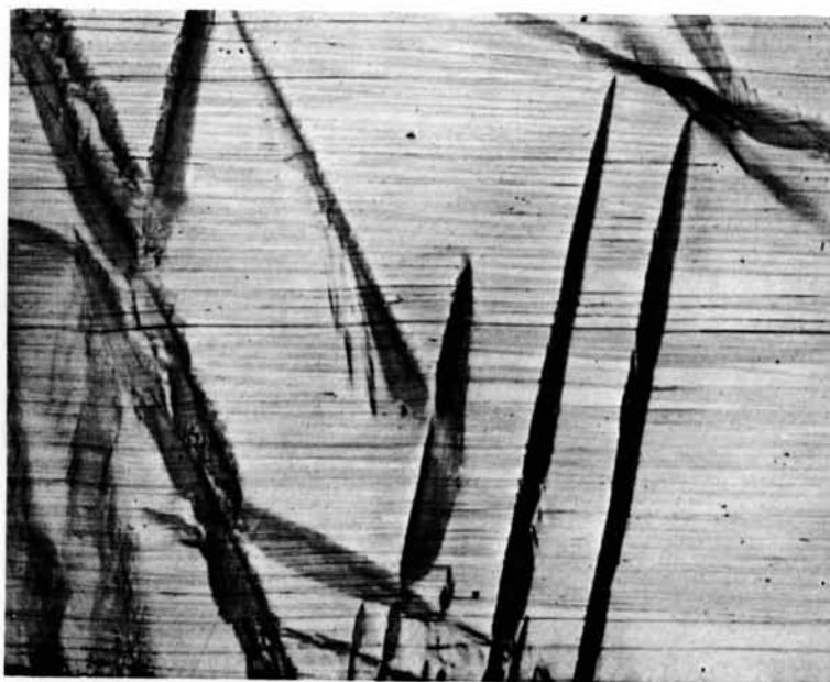
Fig. 10. Photomicrograph showing the manner in which scratches on a polished surface are bent by the production of martensite plates. Specimen is a 30% nickel-iron alloy. \times 150 .
